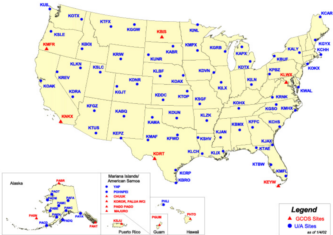
Map of National Weather Service rawinsonde (balloon) network. Blue circles are upper air sites and red triangles are Global Climate Observing Sites.
