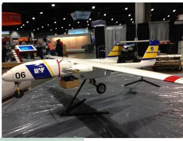
Counter-rotating propellers, heated pitot tubes, fuel injected engines, battery-warmers, and insulation
